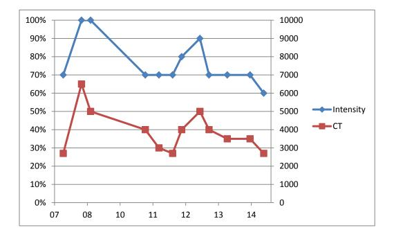
**Figure 1** Continuous changes of intensity and color temperature. The straight lines have the same slope all the way between a particular pair of adjacent control points i.e. a continuous gradual change. The goal for this automatic control is to avoid sudden changes.
