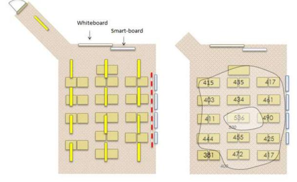
Figure 8 Luminaire position and resulting light distribution.
