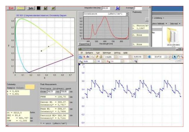
**Figure 33** Simultaneous measurement of calculated light parameters, e.g. colour temperature (ct) and Colour Rendering Index (CRI), and ms light variation.
