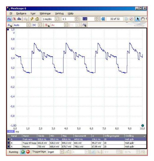
Figure 31 Light variation pattern for one luminaire. Screen dump with time scale 1 ms/division and relative variation of the illuminance, on the y-axsis.
