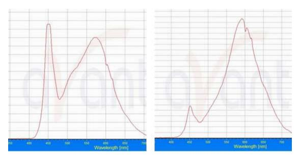
Figure 19 Spectral distribution for the Activating light to the left (The spectrum has a top at 450 nm) and the Dialogure light to the right
