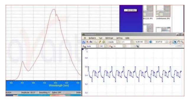
Figure 22 Simultaneous measurement of spectral distribution and ms light variation.
