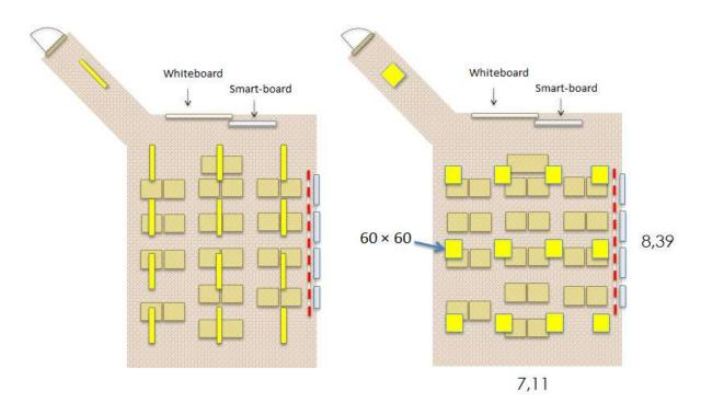
**Figure 10** The plan to the left show the luminaire layout for the old fluorescent tubes. The plan to the right show the new luminaire layout for the 60 × 60 LED panels from Candelux.
