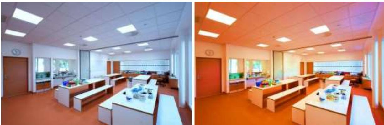
**Figure 20** To the left, cold white light to be used in the morning and during tests. To the right, warm white light to be used e.g. during story time.
